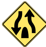
Divided Highway (Road) Ends
