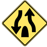
Divided Highway (Road) Ends
